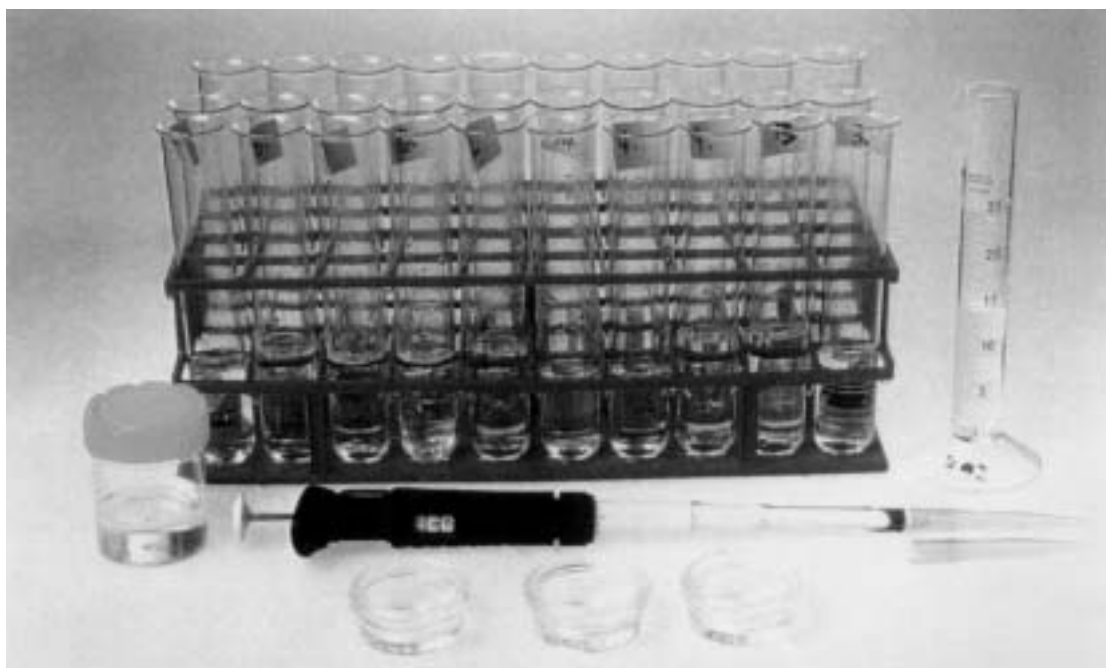
Figure 5. Equipment required for counting nematodes. In the background is a rack with test tubes containing nematodes in water. Alternatively on the far left, a small sample vial can be used for storage of nematodes with minimal water. Far right is a measuring cylinder used to quantify the volume of the sample to be counted. Front centre is a pipette which is used to measure accurately an aliquot of the total sample. This aliquot is placed in the modified Doncaster dishes, three of which can be seen in front of the pipette. These each contain concentric circles and usually hold a 1 ml aliquot of the sample.
